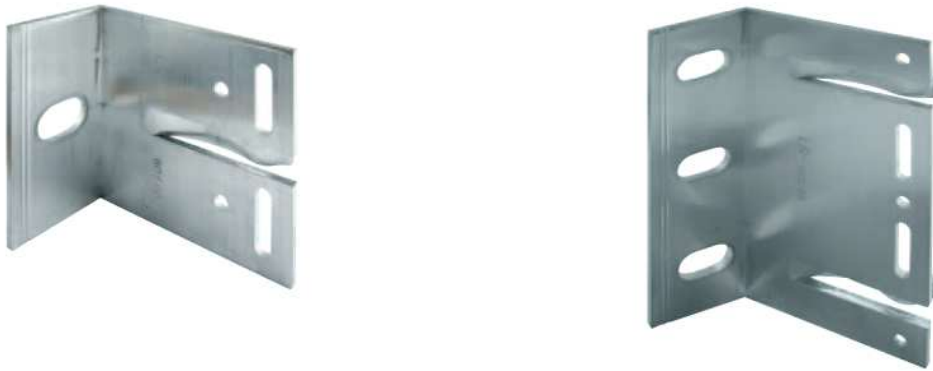
Figure 2.1.6 - Aluminium support brackets Alloy: 6060 T5, minimum thickness: 3 mm
