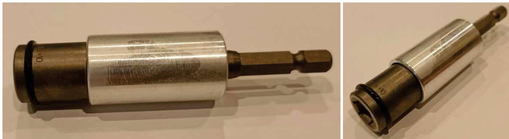
Figure 2.2.19 - Tool for driving the anchors into the Viroc panel
