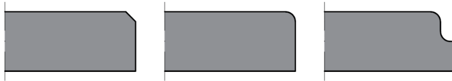
Figure 1.10 - Bevel, groove and notch.
