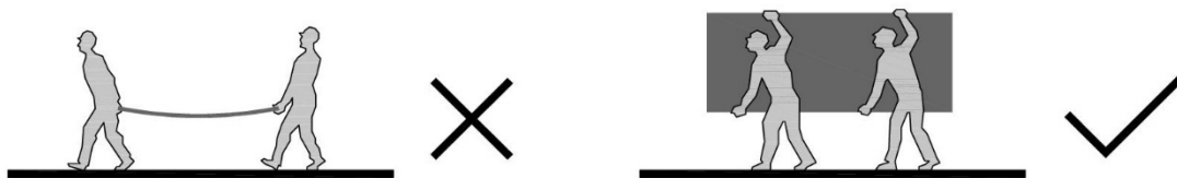
Figure 1.14 - Viroc panels Handling
