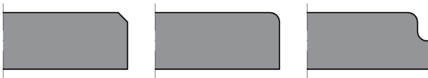
Figure 1.10 - Beveling, rounding and notching.
