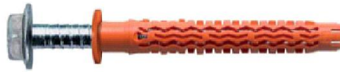
Figure 2.3.5 - Ø10 mm Plastic anchor Stainless Steel or Galvanised Steel Screw Ø7mm, minimum length 75 mm
