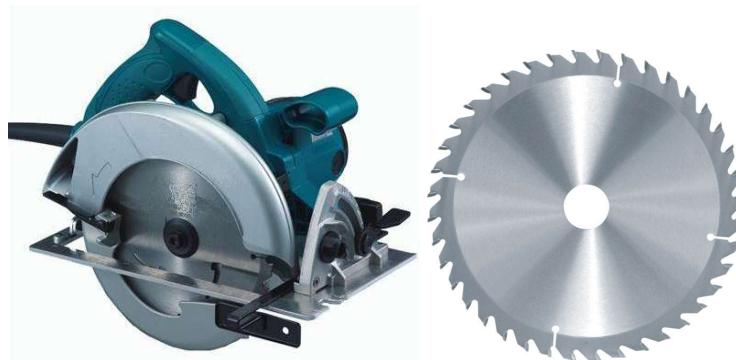
Figure 2.3.16 – Circular saw with tungsten cutting disc
