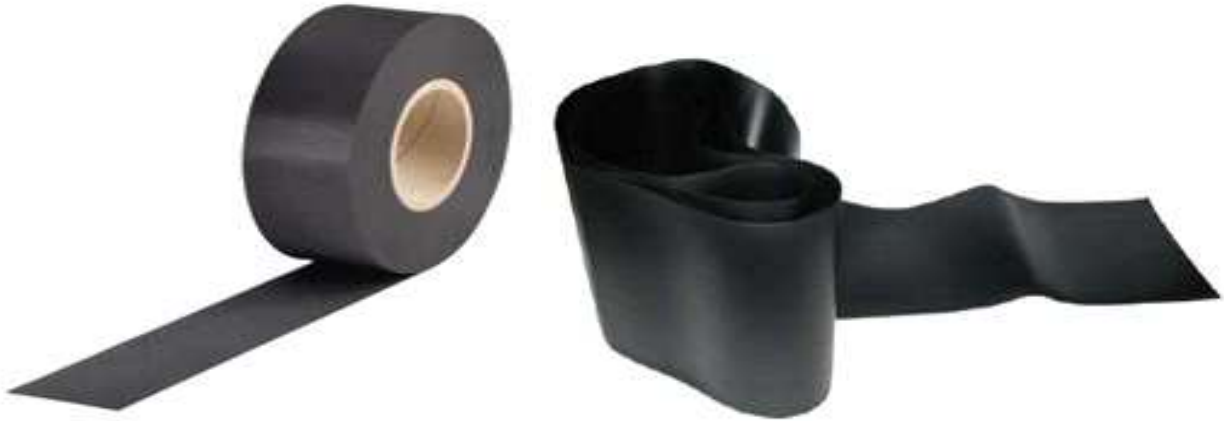
Figure 2.3.8 - Flexible PVC or EPDM protection strip Mandatory on timber studs with durability class 2
