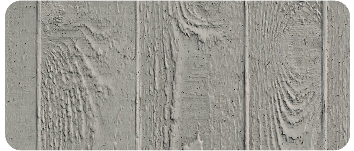
122 Brettschalung | timber formwork
