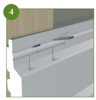
When fastening siding, always press the board firmly against the furring strip. Staples must be positioned directly along the fastening line indicated on the board's profile. Installing the staple above this line may cause the tongue to crack. Staples installed below the line will be visible on the wall.
