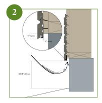
siding and the building; please refer to local building codes to verify ventilation duct guidelines. The ventilation duct must be open and unobstructed to encourage air circulation. The bottom edge of the starter trim should project 1/2" (12 mm) below the bottom of the furring strips. See attached picture.
