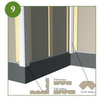
When you install siding next to the corner trim, remember to cut end-joint off and paint the resulting bare wood with touch-up paint.
